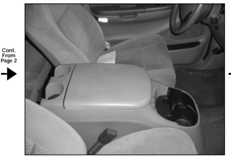
STEP 19: Reinstall console top (removed in Step 5) and place supplied tray into console.
